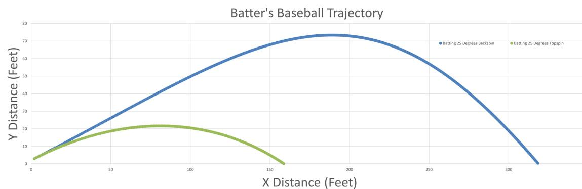
Figure 4: Magnus force simulation of a BATTED baseball (25 degrees) spinning at 6160 revolutions per minute, with both top (158 feet) and backspin (318 feet). The baseball with backspin yielded 157 more feet in the x-direction. These calculations were taken at 760 mmHg (sea level).
