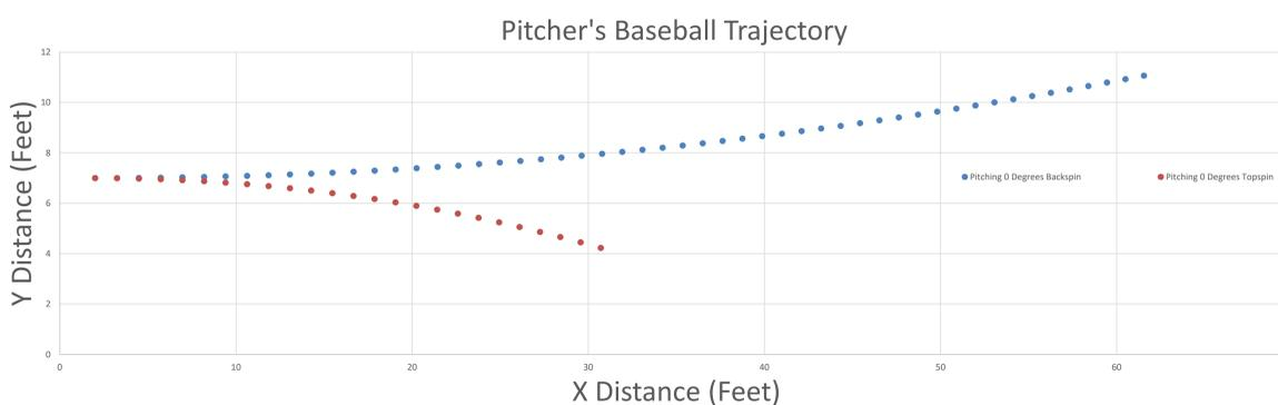
Figure 5: Magnus force simulation of a PITCHED baseball spinning at 6160 revolutions per minute, with both top and backspin. The baseball with backspin rose vertically, corresponding to a pitch named 'riser'. Secondly, the ball with topspin landed before the plate, which is considered a 'curveball'. These calculations were taken at 760mmHg (sea level).
