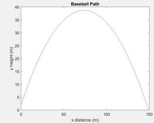
Figure 2: Ball thrown at 45-degree angle at a velocity of 38 m/s (85 mph). This figure refers to a baseball **without** air resistance. Final landing - 149.04m in the x-direction.
