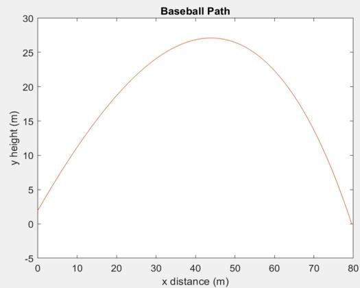
Figure 1: Ball thrown at 45-degree angle at a velocity of 38 m/s (85 mph). This figure refers to a baseball **with** air resistance. Final landing - 79.59m in the x-direction.
