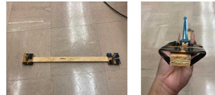
Fig 8: full body of muon telescope (left) and a close up of one of the detectors on the telescope
