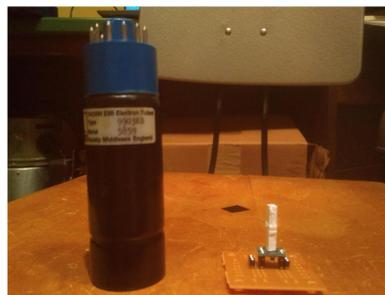
Fig 1: An SiPM (right) and a PMT next to each other
