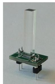
Fig 2: An SiPM with a LYSO crystal on a pin adapter board
