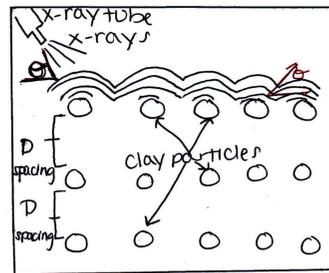
Figure 3. Schematic diagram X-ray Diffractometer. The diffractometer operates under Bragg's Law:  $n\lambda = 2d\sin\theta$  where n reflection number,  $\lambda$  wavelength of the diffractometer, d is the space between layers and  $\theta$  is the angle between the x-ray beam and the layer surface.
