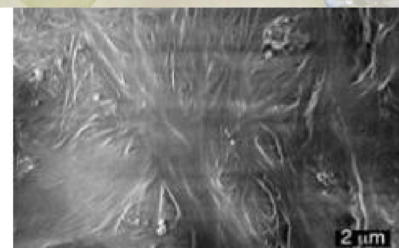
SEM image of xerogel formed from gel of 1 wt % 4 in toluene.
