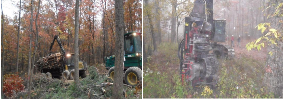
Figure 5: Photo of two forwarders (left) removing logs from the harvest area; and a photo of a processor head (right) that cuts each log to a desired size, delimits it, and spreads out its logging slash evenly across harvest site.
