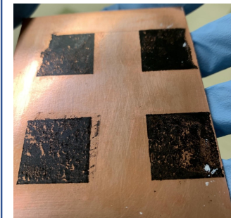
Printing toner, ironed onto a sheet of copper
