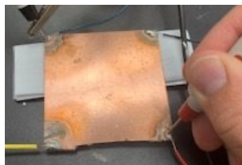
Measuring resistance conventionally with a voltmeter and low-ohm contacts
