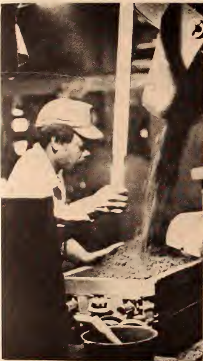
A MOLDER MAKING A SAND MOLD
